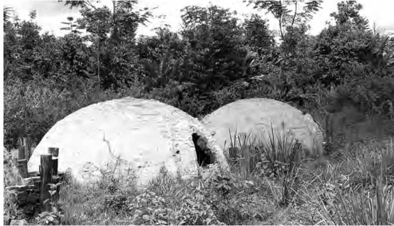
Marabá, Pará, Brazil: charcoal burning to produce charcoal for iron smelting. In spite of the law, there are many illegal facilities
